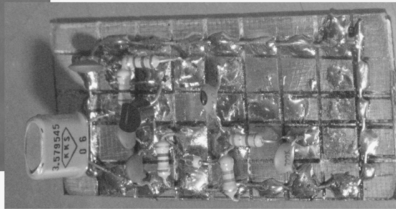
Below The circuit board using pads cut into board with a hack-saw.
