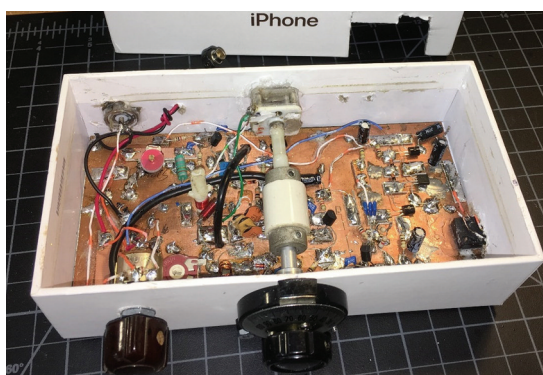
A ceramic DC receiver in an iPhone box
